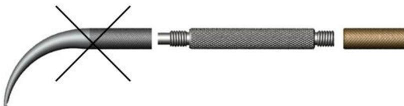
2. Loosen the new (8397) Male Removal Tool a full 3 turns counter clockwise (you will see a visible gap).
