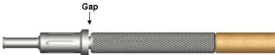
3. To remove a LOCATOR nylon male from the titanium metal housing; simply insert the new tip into the cap/male assembly and push straight in to the bottom of the nylon male. Then tilt the tool so that the sharp edge of the tip will grab hold of the male and pull it out of the cap.
